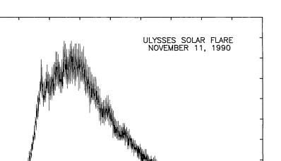
FIGURE 1. Solar flare X-rays observed by the GRB detector on November 11, 1990. The peak occurs around 04:30 UT. Due to the fact that the detector axis points towards the Earth, and the Earth-Ulysses-Sun angle was large, 10-s spin modulation can be observed in the time history.
