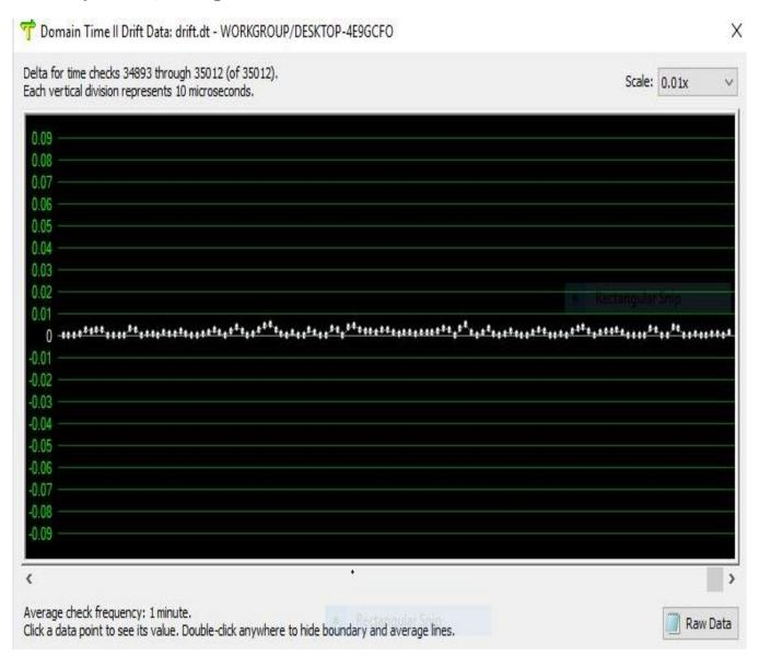
The chart above is an actual example of the computer clock drift corrections to maintain a near zero average microsecond accuracy at the K4LED observatory feeding three Windows 10 computers.
