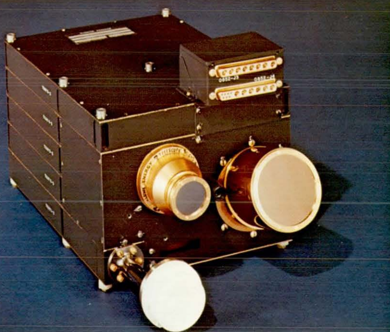
Figure 4-4. Charged particle detectors are used to study the life history of cosmic rays in the Solar System.
