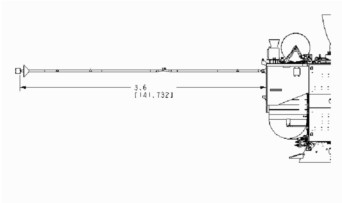
**Figure 3 Magnetometer Deployment.**
