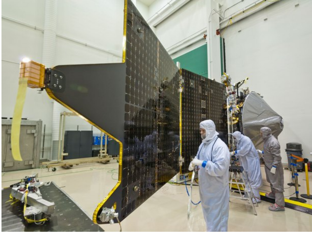
Figure 2: The MAVEN MAG at the end of the MAG boomlet
