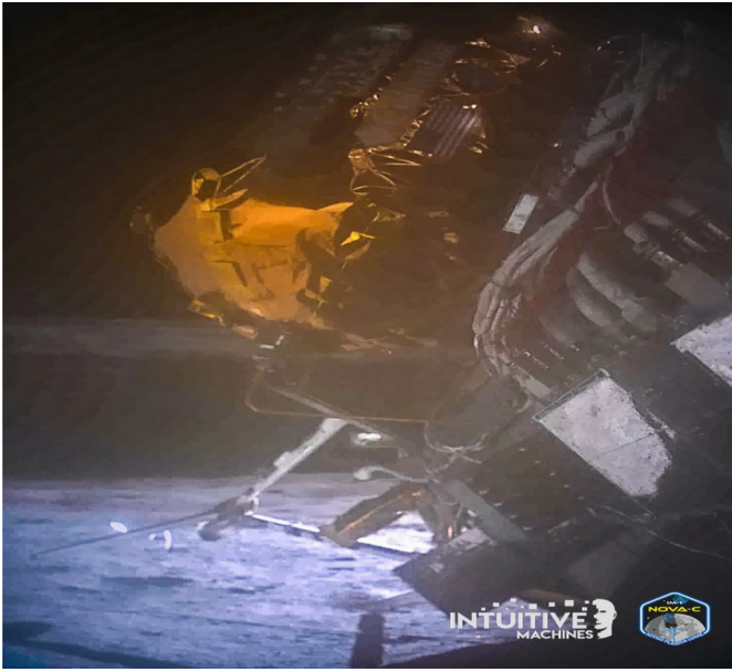
Figure 1. The left panel shows the final image of Odysseus transmitted back to Earth, where the clear tipping of the spacecraft relative to the lunar surface can be seen (image credit to Intuitive Machines). The right panel shows a three-dimensional projection (in arbitrary units) of the Odysseus lander upon the lunar surface, with north and west relative to the Moon’s local topography. The ROLSES-1 antennas are labeled from A through D, shown as blue lines with red labels. Odysseus most likely lays upon its northwest panel, crushing antenna D beneath it. The lunar surface slopes up to the north at an angle of 12^\circ . The exact height of Odysseus above the lunar surface is not known, and the attitude angles (yaw, pitch, and roll) all have 5^\circ errors.
