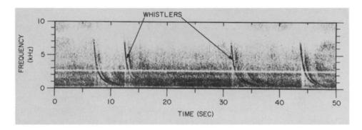
Fig. 8. A frequency-time spectrogram made up using an S<sup>3</sup>-A lightning whistler recording as input for the Voyager PWS broadband channel. The horizontal line is present because of the action of the PWS notch filter.
