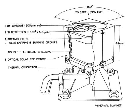
FIGURE 5. The soft X-ray detectors. The two Si surface barrier detectors point towards the Earth. Inflight calibration is provided by two 20-nCi <sup>129</sup>I sources.
