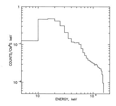
FIGURE 6. Background spectrum from one of the hard X-ray detectors, taken in the calibration mode. The 60-keV <sup>241</sup>Am peak is visible.
