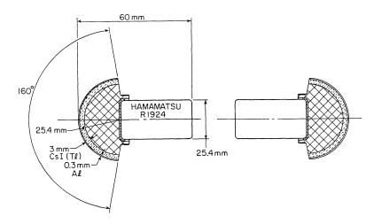
FIGURE 4. The hard X-ray detectors. The axis points towards Earth. Each unit contains a 10-nCi <sup>241</sup>Am source for inflight calibration. The energy resolution is about 40% at 60 keV, and the noise threshold around 10 keV, in the laboratory at ambient temperature.
