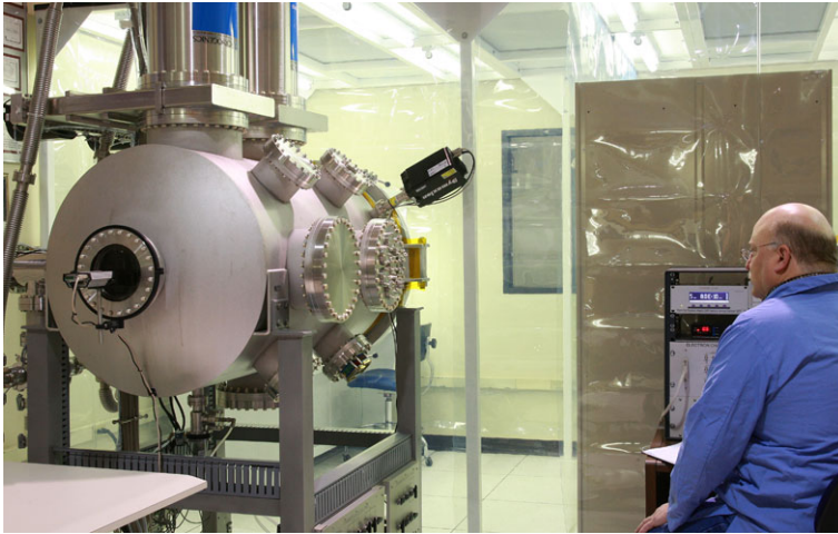
Fig. 83 The Southwest Research Institute Electron Calibration Facility. The main vacuum vessel has an approximate volume of 580 liters. Access to the interior of the chamber is through a Viton sealed door inside a class 10,000 clean tent, which includes a class 100 clean bench to facilitate final work on the instrument prior to installation into the vacuum chamber. Vacuum feed throughs of varying sizes circle the chamber and are accessible outside the clean tent
