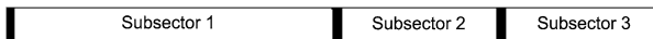
Fig. 27 Structure of the rotational (and timing) subsectors in the JEDI data accumulation scheme that allows us to sub-commutate in a flexible manner between the 3 different species collection modes: electron spectra, ion spectra, and ion species. One can choose to use a cyclic of combination of modes within these subsectors. There are 60 sectors per spin, and so this pattern of subsectors occurs 60 times per spin
