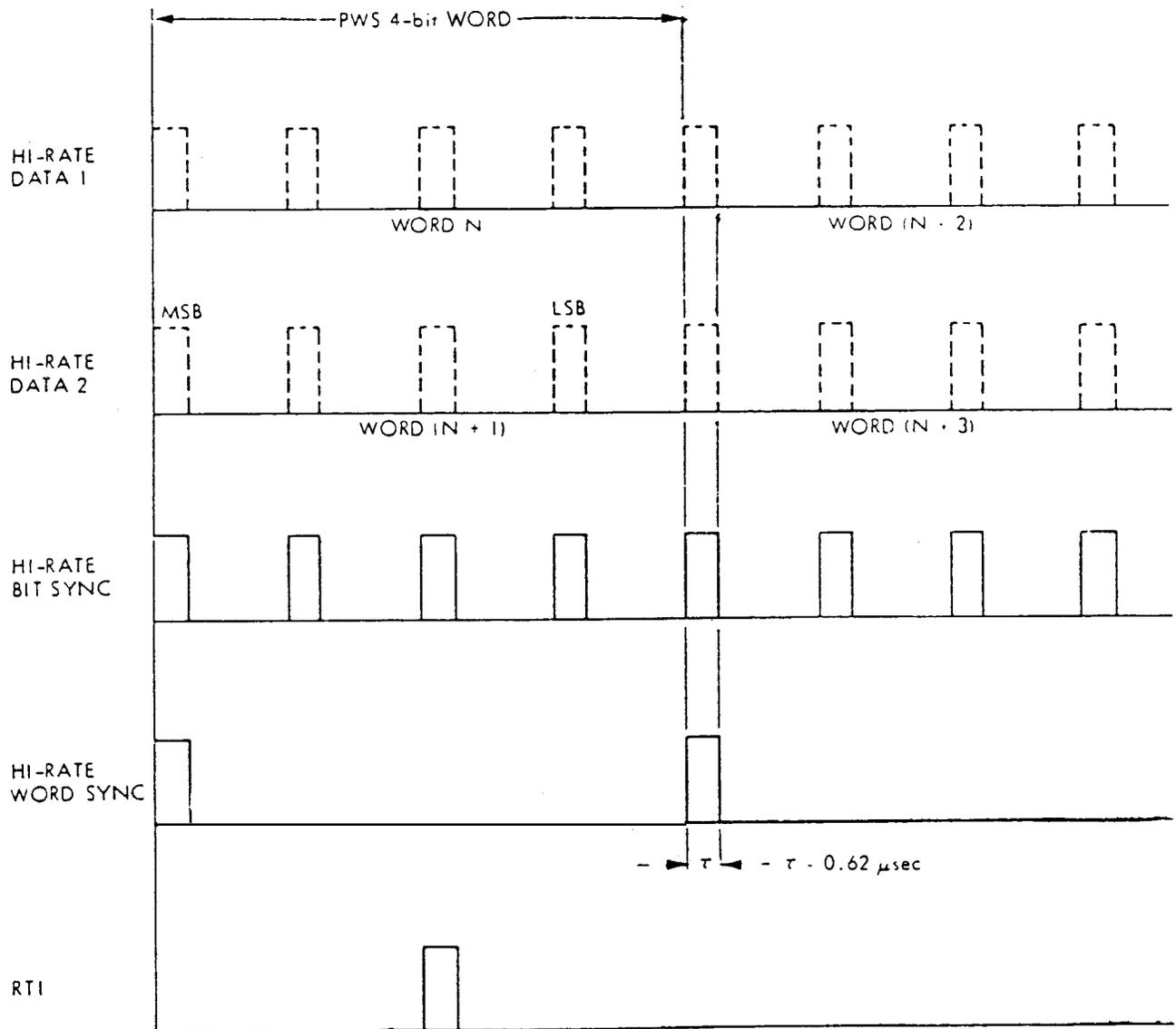
NOTE: ALTERNATE 4-BIT WORDS ARE CLOCKED ON PARALLEL DATA LINES
