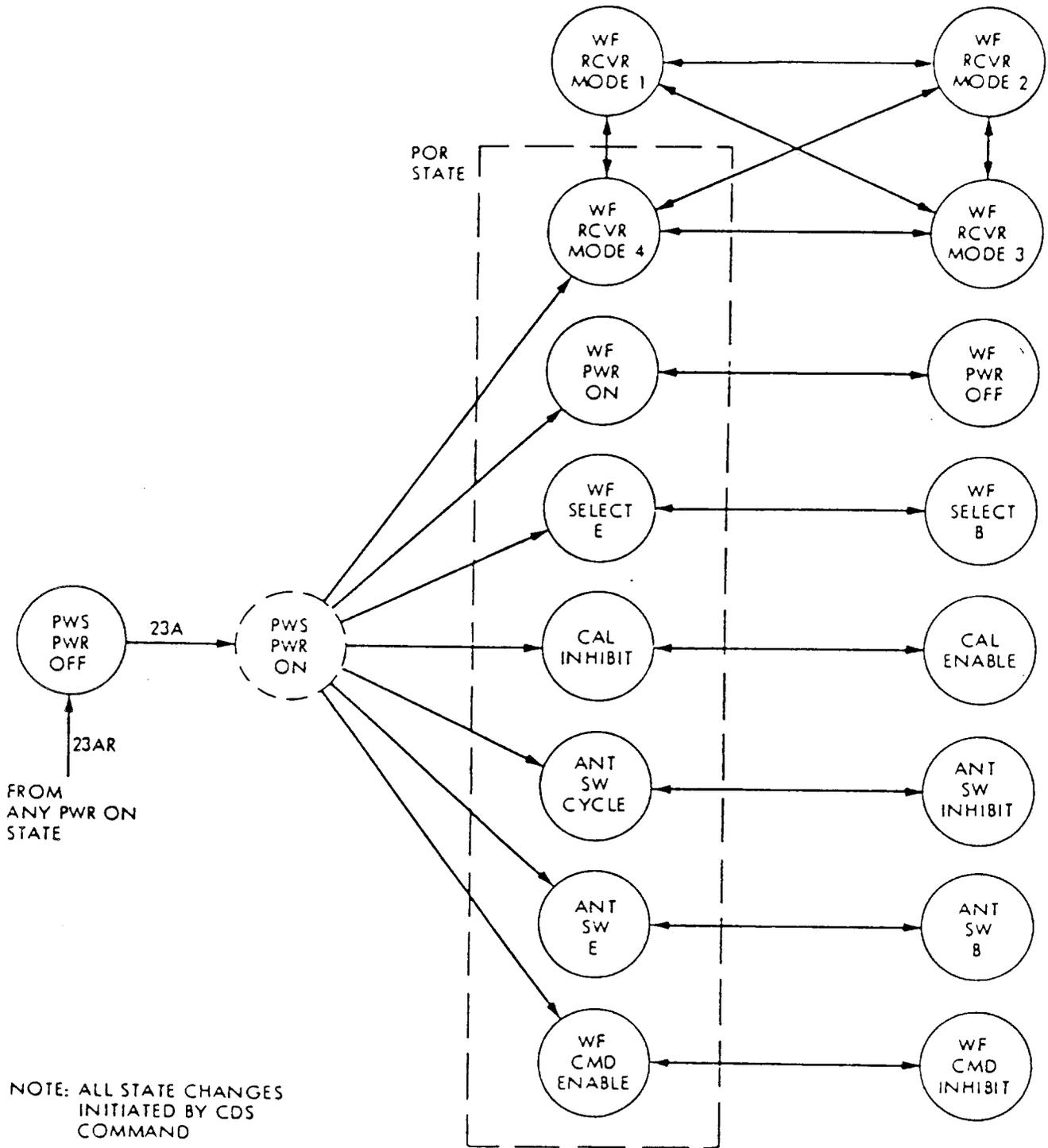
Figure 5. PWS State Diagram
