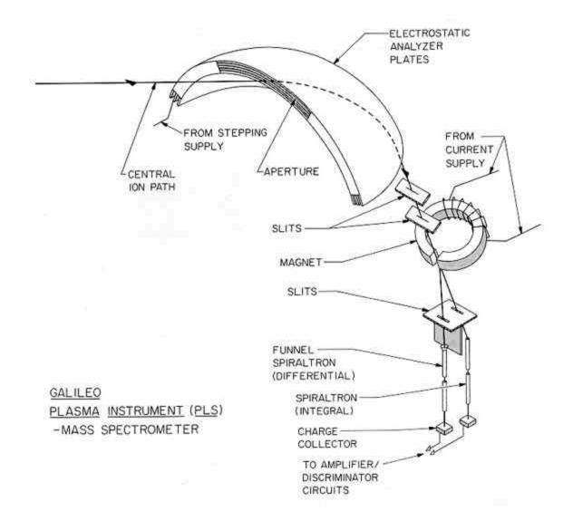
Fig. 5 . Configuration of one of the three miniature, magnetic mass spectrometers in the plasma instrument.
