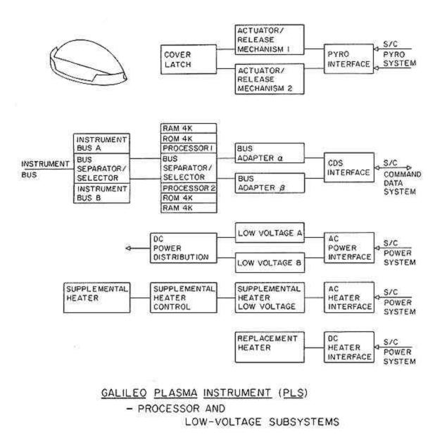
Fig. 10. Block diagram for the electronics in the plasma instrument. Two microprocessors are used to improve the reliability.
