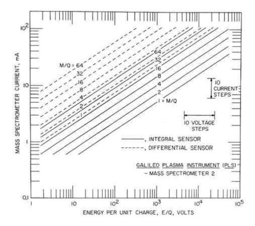
Fig. 7. The relationship of energy-per-unit charge (E/Q), mass spectrometer current, and massper-unit charge (M/Q) for the detection of positive ions with the miniature mass spectrometers. The E/Q value is 960 V for a corotating  $S^+$  ion at equatorial radial distance 6  $R_i$ , in the Jovian magnetosphere.
