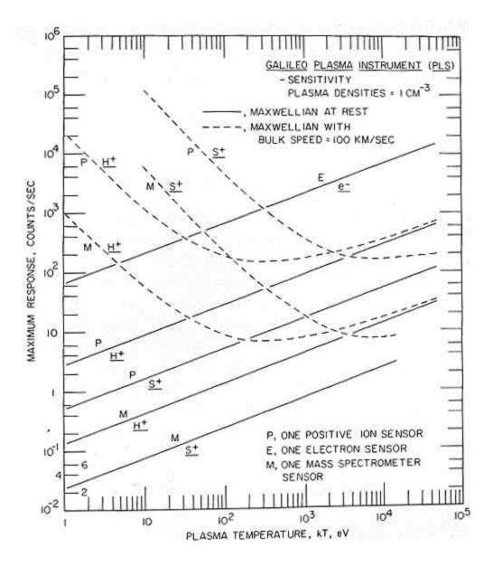
Fig. 8. Maximum responses of several individual sensors to a Maxwellian plasma distribution as a function of plasma temperature. Responses to  $H^{+}$  and  $S^{+}$  plasmas at rest and with bulk flow speed 100 km s<sup>-1</sup> are shown. The densities of electron and ion plasmas are each taken as 1 cm<sup>3</sup>.
