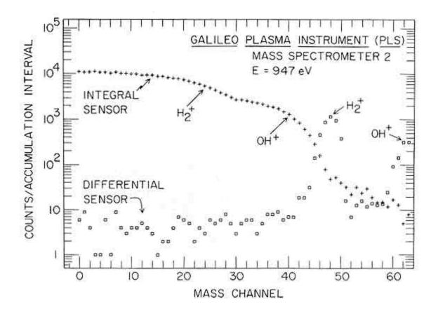
Fig. 6. Calibration of a miniature mass spectrometer with an ion beam  $(H_2^+, OH^+)$ . The unresolved water group  $(O^+, OH^+, H_2O^+)$  is designated as  $OH^+$ . The beam energy is 947 eV and the beam current is constant. The responses of the integral and differential channels are shown as a function of electromagnet current (mass channel). The current increases by a logarithmically equal increment for each mass step.
