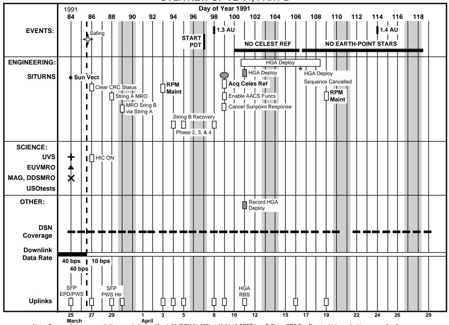
Note: Spacecraft sequence activities were halted on March 26 (DOY 91-085) at 13:31:18 SCET by a B-String CDS Bus Reset, which resulted in spacecraft safing. Except for brief RBS sequences, the spacecraft was under real-time control until the start of EE-2' on Sept. 3, 1991 (DOY 246).
