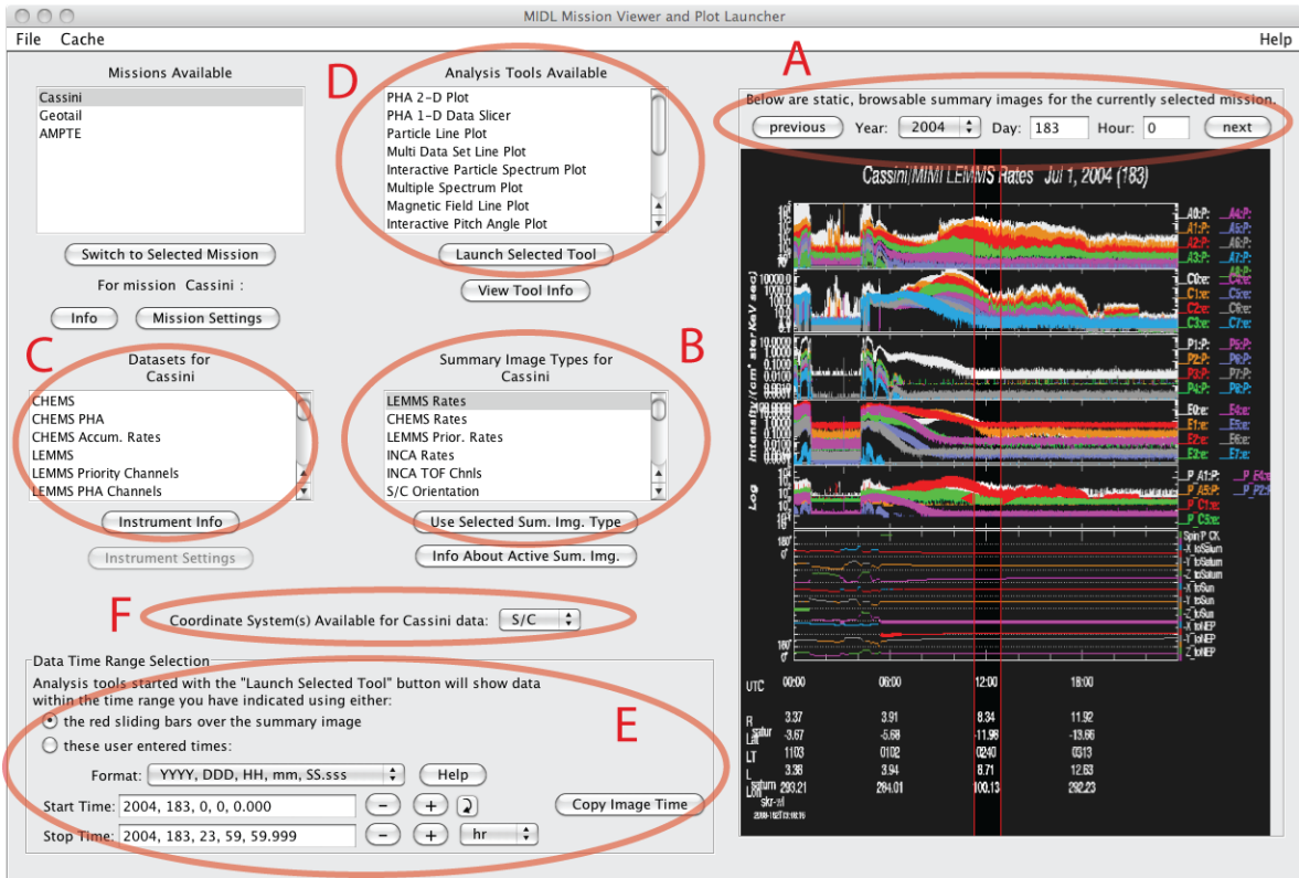
Figure 6.2: The main screen of MIDL. Pre-made summary plots are shown on the right as a quick way to explore the data. The left panel offers options for choosing data to view and the tool with which to view it. Key features are circled and labelled A through F. Feature A is the time range selector for the summary images. There are many different types of pre-made summary images, and the summary image selector (B), lets you choose the one to view in the right panel.
