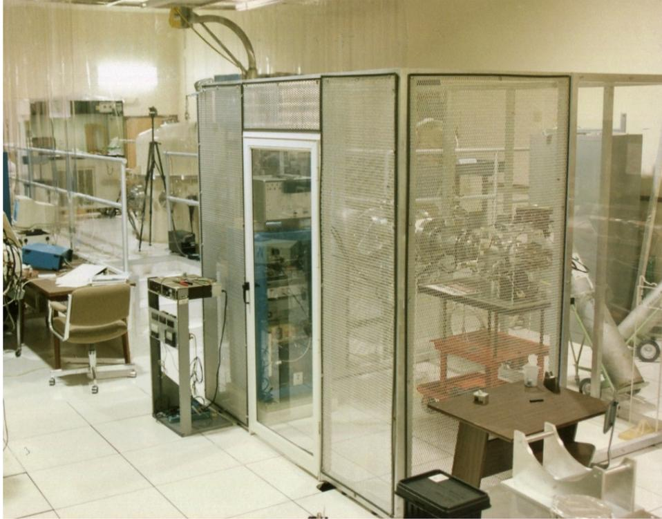
**Figure 8. IBCS high voltage Faraday cage with ion source inside. The vacuum chamber is at the far end of the room in this photo.**
