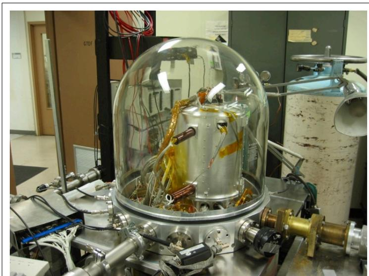
Figure 4 showing PM IMS in bell jar chamber that is attached to the beam line of the Medium Energy Accelerator Facility at GSFC in Bldg. 22.
